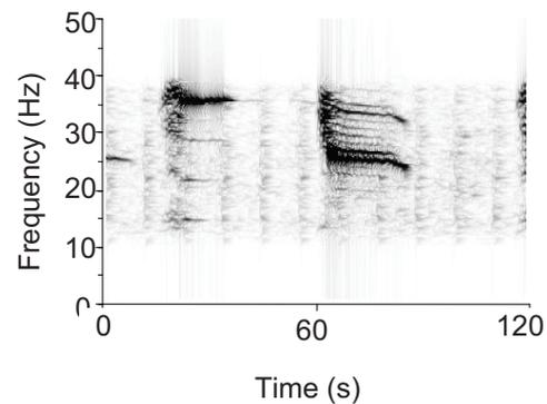
**Figure 2: Spectrogram of pygmy blue whale calls “Madagascar type” recorded off Crozet Island (Spectrogram parameters: 1024 points FFT length, 90% overlap, 250 Hz sample rate, Hanning, for a filter bandpass between 12 and 40 Hz).**
