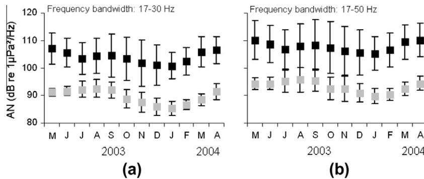
**Fig. 4.** One year of ambient noise level received at the Northern array (grey) and at the Southern array (black) in the frequency bandwidth of Antarctic blue whale calls (a) and pygmy blue whale calls (b) in the Southwestern Indian Ocean.
