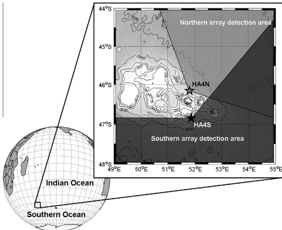
**Fig. 1.** Location of the two arrays (grey stars: Northern array and black star: Southern array) of the hydroacoustic station of the International Monitoring System moored in the Southwestern Indian Ocean near Crozet Islands. The potential call detection area for the both arrays (grey area: Northern array and black area: Southern array) is delimited from the detection range modeling using the Range-dependant Acoustic Model.
