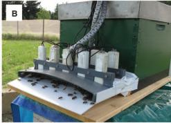
Fig. 1. Honey bee RFID monitoring equipment. (A) A pollen-forager honey bee fitted with a 3-mg RFID tag. (B) A hive entrance equipped with RFID readers for detecting returning marked foragers.
