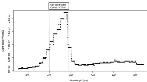
**Figure 3.** Spectral range of the photodiode included into the TDR10-X. [Color figure can be viewed at [wileyonlinelibrary.com](http://wileyonlinelibrary.com)]
