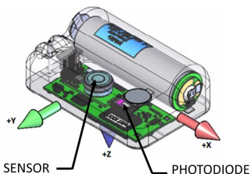
**Figure 1.** Schema of a TDR10-X with the different axis orientation: *x* from left to right, *y* from backward to forward and *z* from top to bottom. (Wildlife computers: <http://wildlifecomputers.com/wp-content/uploads/manuals/MK10-User-Guide.pdf>).
