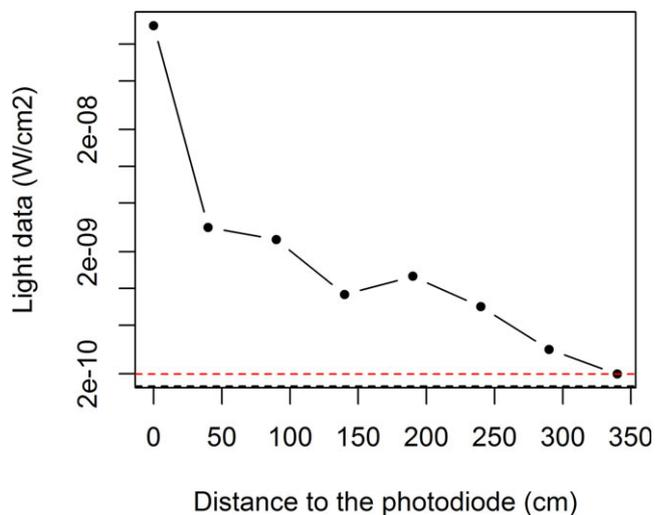
**Figure 5.** Distance of detection of the photodiode included into the TDR10-X. A 465 nm blue LED with an intensity of 700 million RLU which corresponds to  $1.2 \cdot 10^{-7} \text{ W cm}^{-2}$  was used in that experiment. The black dotted line corresponds to the darkness condition, and the red dotted line corresponds to the darkness condition to which was added the measure precision.
