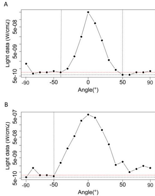
**Figure 4.** Detection angle of the photodiode included into the TDR10-X. Graphs A and B represent, respectively, the detection angle of the photodiode on the x-axis and y-axis. The black dotted line corresponds to the darkness condition, and the red dotted line corresponds to the darkness condition to which was added the measure precision.
